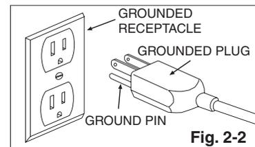
**Important:** This product is for use on a standard 120-volt AC circuit and has a grounded plug like the plug in Fig. 2-2. If it does not fit the receptacle, have a proper outlet installed by a qualified electrician. DO NOT modify the plug provided with this product.
